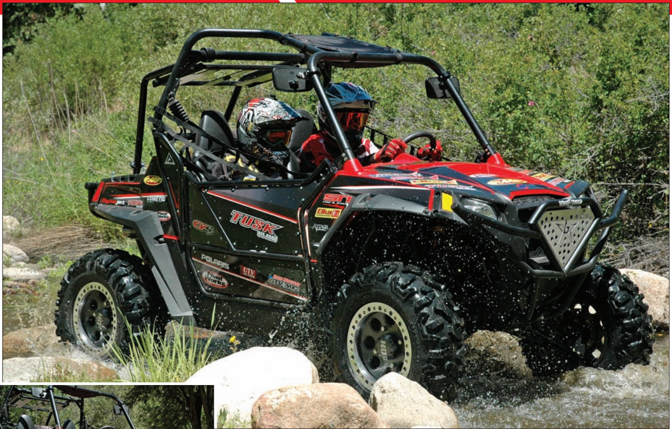
Tusk aluminum doors with custom Attack Graphics replaced the annoying stock nets. STI Roctane XD tires on STI HD beadlock wheels keep the RZR rolling in style no matter how tough the terrain gets.
