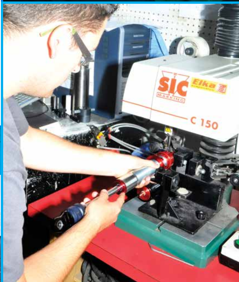
ONCE A SHOCK IS APPROVED BY QUALITY CONTROL IT IS ENGRAVED WITH ITS UNIQUE SERIAL NUMBER
