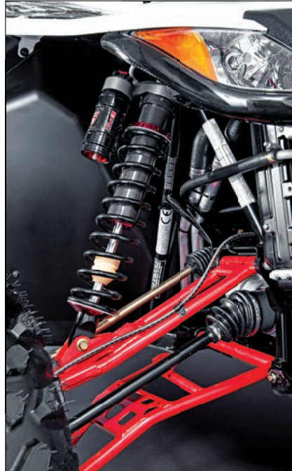
Base and XT versions sport the JRi EXC-1 shock with 70-position compression adjusters, while the LTD EPS has Elka Stage 5 piggyback shocks with high- and low-speed compression clickers, plus rebound and ring preload. Check out the double-row, high-capacity radiator, which has a thermostat-controlled fan.
