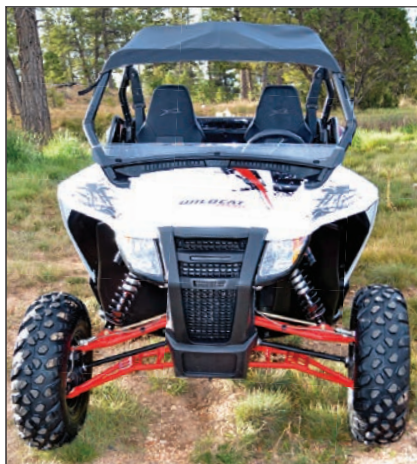
Front travel is 12.2 inches with either shock package, and tires are 26-inch Carlisle Trail Pros. Halogen headlights grace all three versions, and ours was equipped with an accessory soft Bimini roof ($119.95) and windscreen deflector ($149.95).
