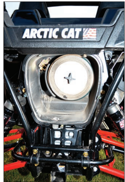
Undo five clasps to access the large, pleated-paper air filter, and the huge still airbox has a handy drain and high-placed intake duct.
