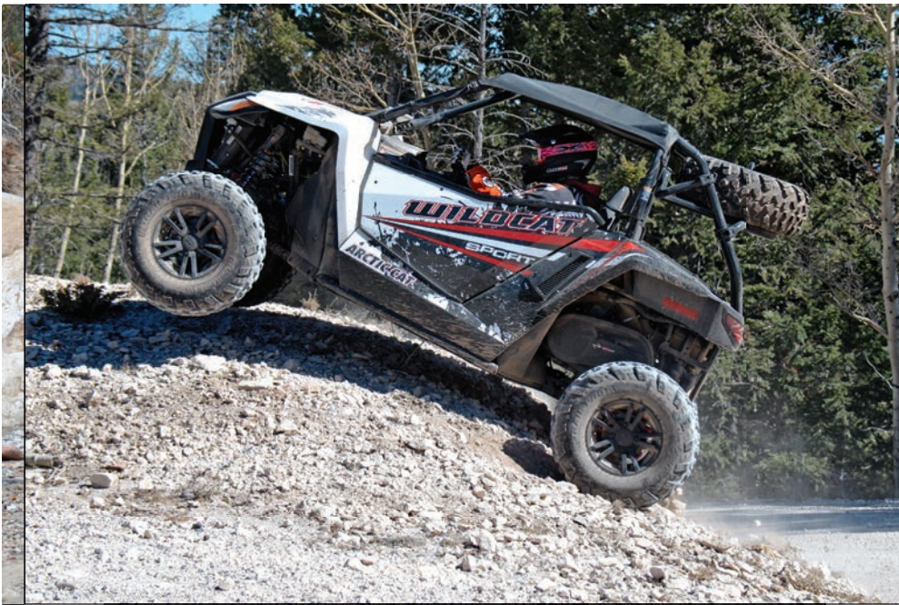
In between the Wildcat 1000 and the 50-inch Wildcat Trail, the new Wildcat Sport fills the 60-inch UTV niche with more than a foot of travel, adjustable piggyback shocks, and an excellent engine and CVT package. It comes in three versions for 2015, with the Limited getting EPS, full doors and fully adjustable Elka Stage 5 shocks.
