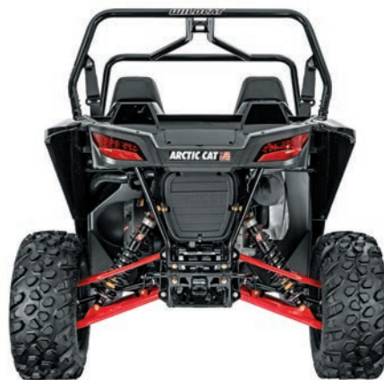
Rear travel is 12.6 inches, and it's rated to tow 1500 pounds with the standard 2-inch automotive-style receiver. A removable panel in the bed allows access to the spark plugs.
