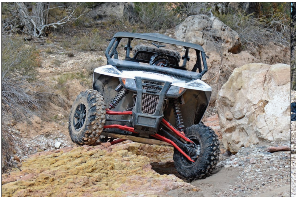
Whereas the Trail Cat has front and rear torsion bars, the Wildcat Sport has one heavy-duty torsion bar in the rear, and the long, gull-wing A-arms provide plenty of articulation for rock crawling. The Sport also has 26-inch tires (but has the horsepower to turn 29s) and 13 inches of ground clearance.
