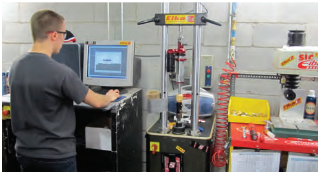
A technician testing a shock on the dyno to ensure it's operating within their specs.
