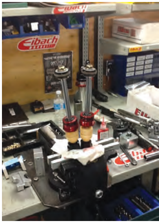
Two shock shafts with valve installed awaiting final assembly.
