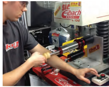
Each shock gets a serial number engraved once it passes all the tests.
