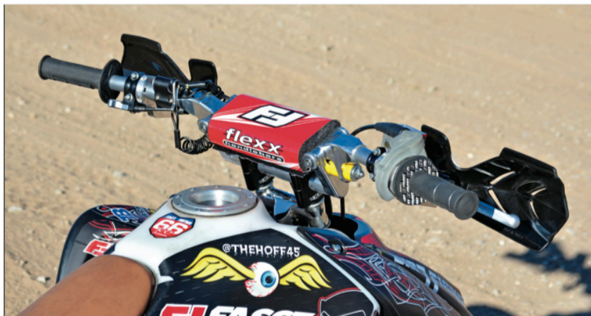
To control the rat rod quad, Colt relies on Fasst Co.'s Flexx handlebar with impact and rebound elastomers. Works Connection handles the levers and hot start.
