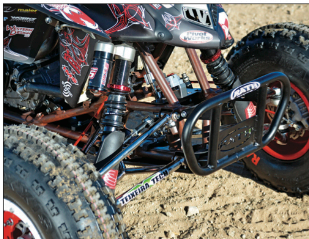
The Teixeira Tech and Elka suspension combo offers extra width and a ton of travel to get through the deepest whoops. A Fastway steering damper helps soften any high-speed, unexpected hits.
