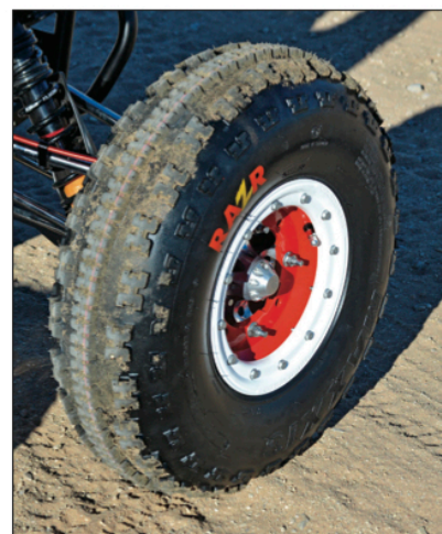
Goldspeed wheels with white beadlock rings give the appearance of having white-wall tires complementing that old-school street-rod look. The Maxxis Razr tires that are used don't come in white walls but are the top choice of many winning desert racers.
