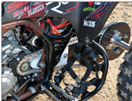
A gnarly set of footpegs and lightweight heel guards is about all Colt uses to stand on. Most desert racers do not use nerf bars as contact with other riders and machines is rare.
