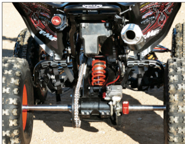
To get the most ground clearance, GNCC and desert guys are running round sprocket guards and disc savers like the one sandwicheing the chain and sprocket on the left side. This one is from CRF.
