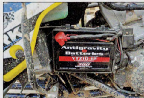
Today's fuel injected quads require a strong battery in good-working condition to power all the electronics. This Antigravity lithium-ion battery does that all while weighing half that of a lead-acid product.
