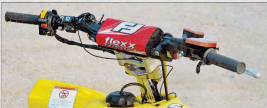
Any little tricks you can do to fight rider fatigue is well worth it if you want to go fast for a long time. These Flexx bars from Fastt Co., along with a GPR stabilizer, attach to the Roll Anti-Vibe stem almost give you the same advantage as installing aftermarket shocks.
